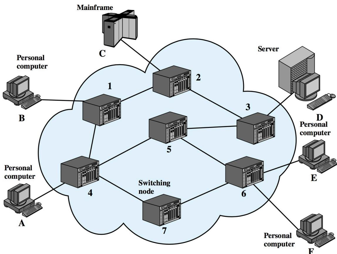
2. Explain datagram Network which uses packet switching with neat diagrams.
