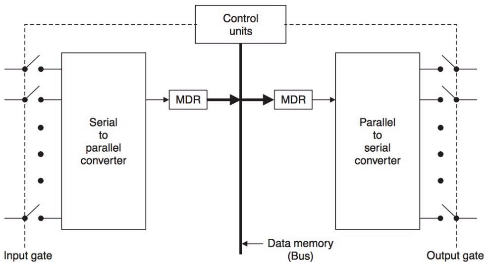
The analog time division switching is useful for both analog and digital signals. The digital time division multiplexed signals usually requires switching between time slots as well as between physical lines.
