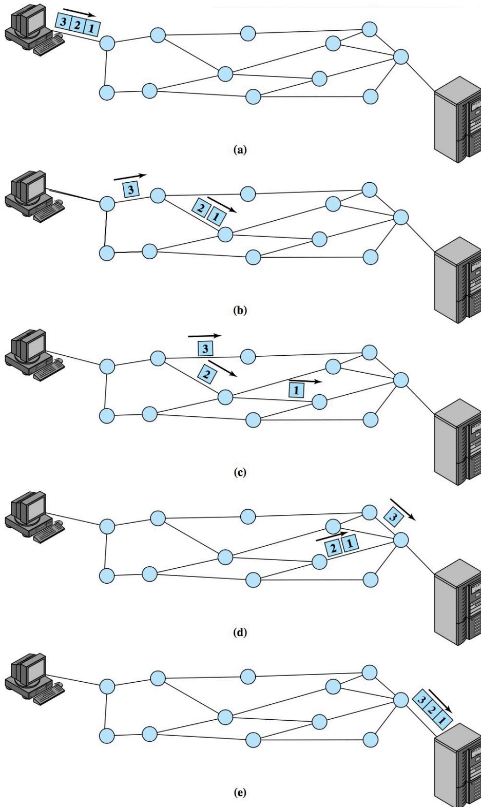
3. Explain Virtual Circuit Connection setup with neat diagrams.
