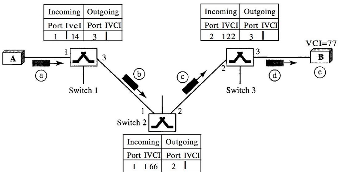
A special frame, called the acknowledgment frame, completes the entries in the switching tables.
