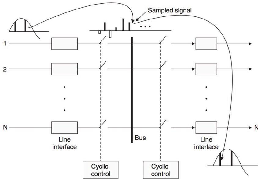
If PCM binary samples are switched, then the switching is known as digital time division switching.
