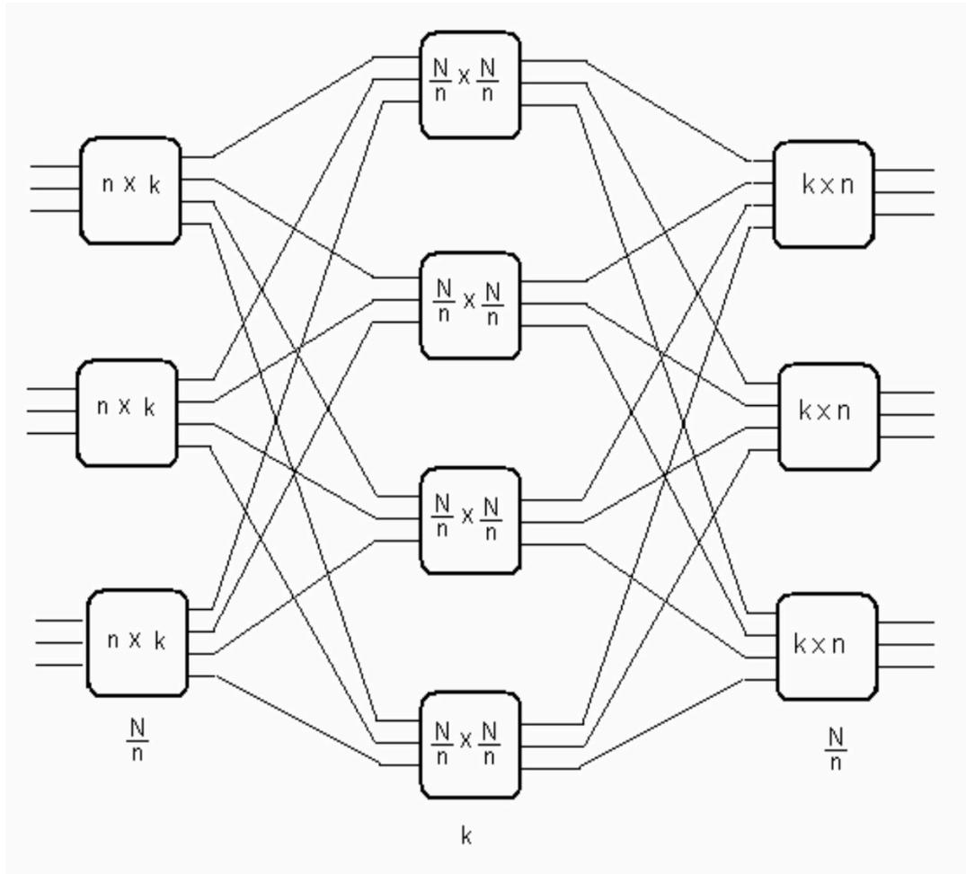
Out of  $N$  lines,  $\frac{N}{n}$  groups of  $n$  lines are made available as input and output.
